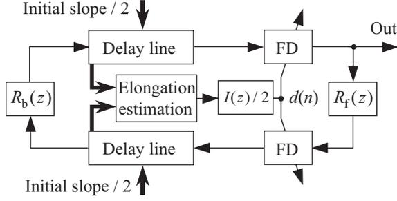
**Fig. 1.** Waveguide string model where elongation caused by string vibration affects the loop delay through modulation of the fractional delay (FD) filters [5], [6]. The input signal is the initial slope that is inserted into both delay lines.
