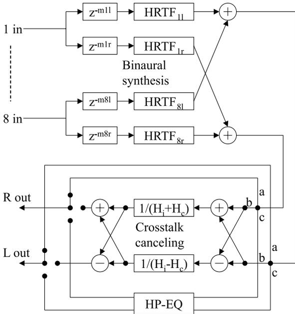
Figure 2: A block diagram of the binaural part of the auralizer. The binaural signal is optionally routed a) directly to the output b) through the crosstalk canceling filters or c) through headphone compensation filters.
