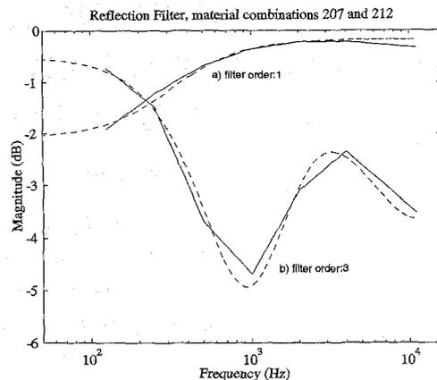
Figure 1: First-order and third-order minimum-phase IIR filters designed to given absorption coefficient data.
