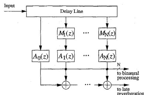
Figure 7: Structure for image-source implementation with reflection and air absorption filters.
