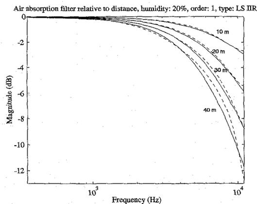
Figure 2: First-order IIR air absorption filters proportional to distance (in meters).
