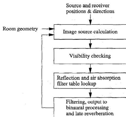
Figure 6: Image-source calculation process in the DIVA system [17].
