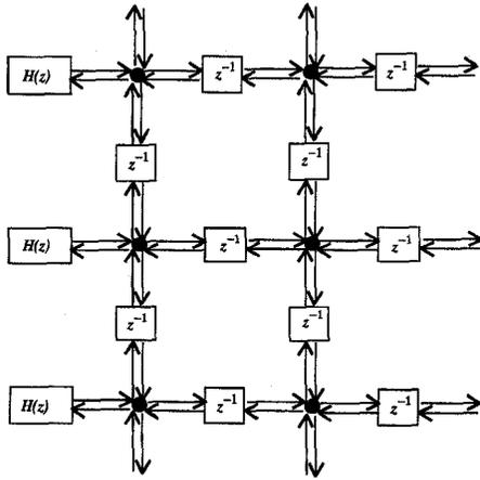
Figure 3: Two-dimensional waveguide mesh structure with boundary filters.
