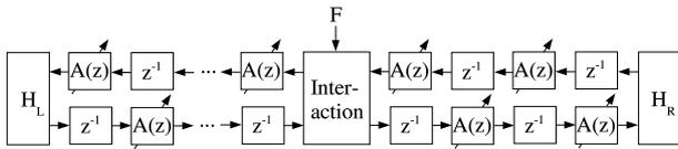
Figure 2: The single-polarization string model.  $A(z)$  denotes an allpass filter, while  $z^{-1}$  denotes a unit delay.  $H_L$  and  $H_R$  are FIR filters modeling the frequency-dependent losses at the left and right string termination points, respectively. The interaction element provides means for inserting a force signal into the string, and its location can be changed.
