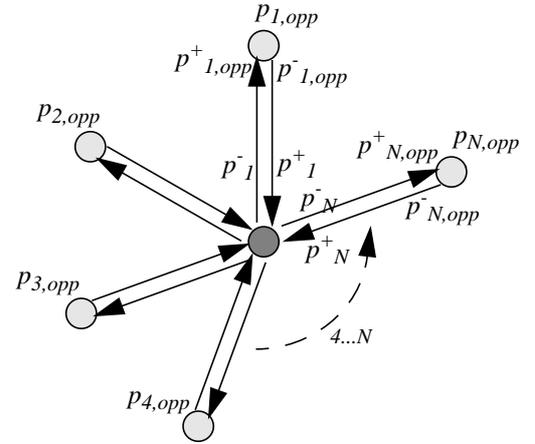
**Fig 1.** A scattering junction with  $N$  neighbors connected by bi-directional unit delay elements.
