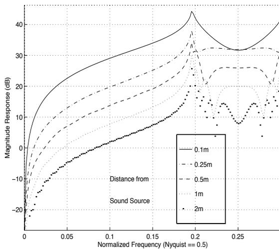
**Fig 3.** Magnitude response registered from various distances at diagonal direction.
