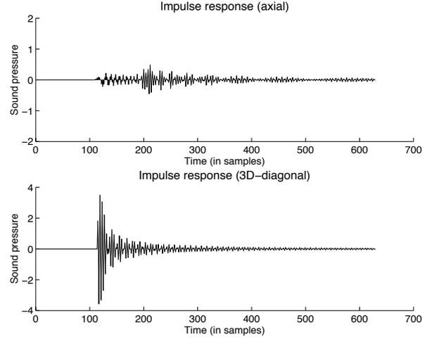
**Fig 4.** Impulse responses to axial and 3D-diagonal directions at the same distance from the sound source.
