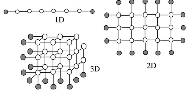
**Fig 2.** Example structures of rectilinear 1D, 2D and 3D meshes.
