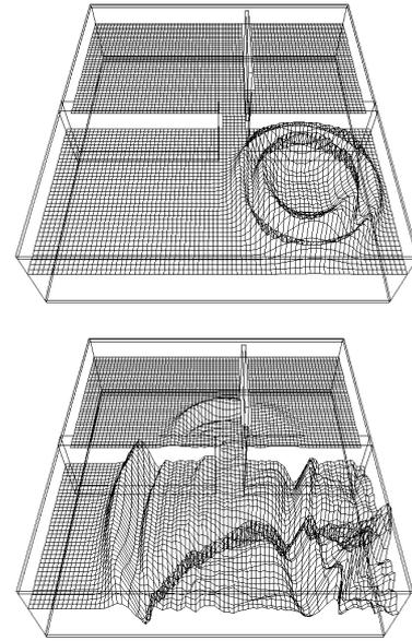
**Fig 7.** Visualization of simulation, excitation and first order reflection (above), wall reflections (below).
