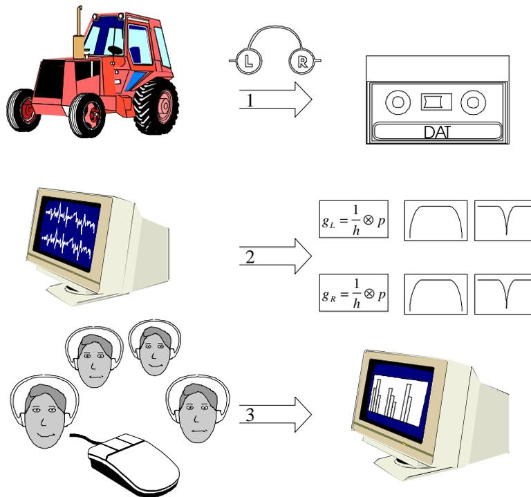
Figure 1. The binaural sound quality evaluation system. The sound samples are recorded binaurally to DAT tape (1). The samples are edited using digital signal processing (2) and presented to many subjects simultaneously in the listening test (3). The subjects give their answers by pressing the mouse buttons. The results are analyzed by statistical means.
