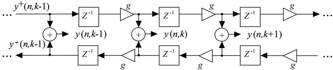
Figure 2: *Lossy digital waveguide. After Smith [3].*
