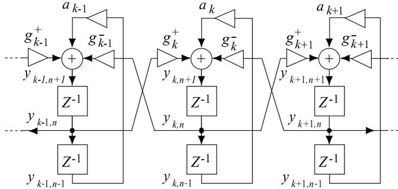
Figure 1: *Digital waveguide structure based on finite difference approximation of one-dimensional wave equation.*
