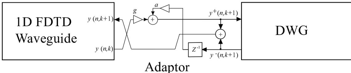
Figure 4: *The adaptor formulation of the corresponding hybrid model.*
