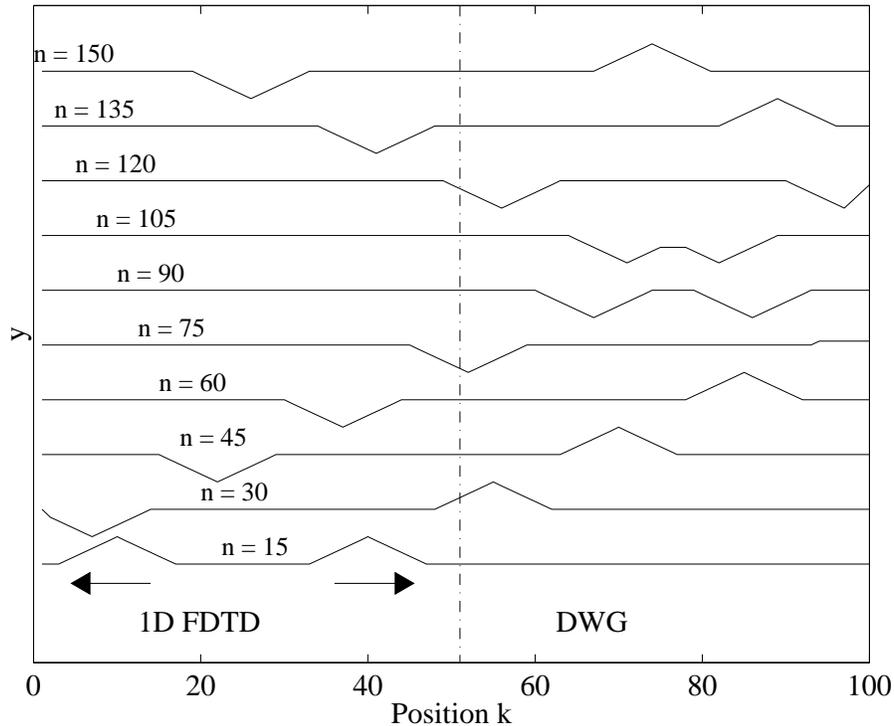
Figure 5: The displacement of the string at various time instants  $n$  as calculated by the hybrid model shown in Fig. 3. The terminations are rigid at both ends. The adaptor is placed at  $k = 51$ . At the instant  $n = 0$  (not shown in the figure) a triangular initial displacement pulse is inserted into the 1-D FDTD side. As  $n$  increases, the traveling components propagate in the hybrid structure.
