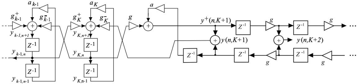
Figure 3: *The interconnection of a 1-D FDTD waveguide to a DWG.*
