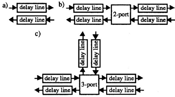
Fig. 2. Block diagrams for the basic digital waveguide elements: a) a digital waveguide, b) a connection of two digital waveguides via a two-port, and c) a connection of three digital waveguides via a three-port.
