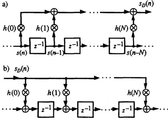
Fig. 3. FIR-type a) interpolation and b) deinterpolation.
