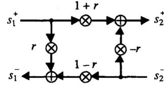
Fig. 4. A 2-port connecting two digital waveguides, like in Fig. 2b.
