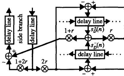
Fig. 6. A side branch connected to a fractional point of a digital waveguide. The input and output of the delay lines are computed using  $N$ th-order FIR interpolation and deinterpolation.
