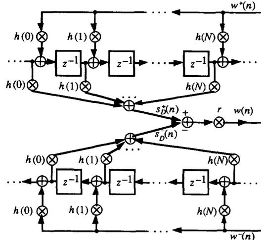
Fig. 5. The fractional delay Kelly-Lochbaum junction implemented using  $N$ th-order FIR interpolation and deinterpolation.
