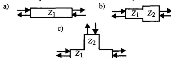
Fig. 1. a) A single waveguide, b) a waveguide junction, and c) a waveguide with a side branch.
