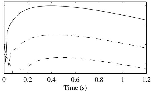
**Figure 4:** Amplitude envelopes of the second harmonic of the synthetic string vibration signal with  $A_{g_{str}} = 0.001$  (bottom curve),  $A_{g_{str}} = 0.002$  (middle curve), and  $A_{g_{str}} = 0.005$  (top curve).
