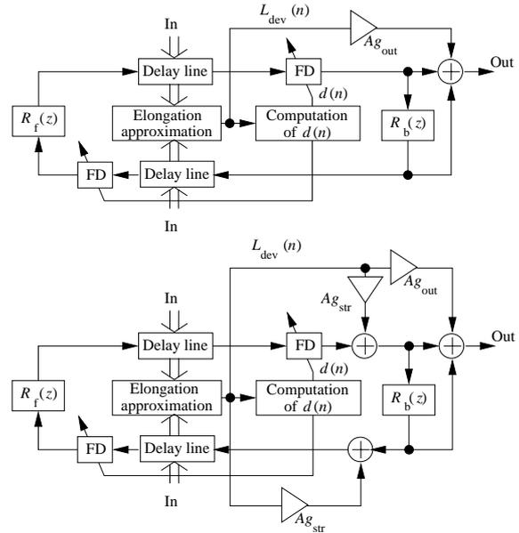
**Figure 3:** Dual-delay-line waveguide model of a string including TMDF output (top), and TMDF output and coupling (bottom).
