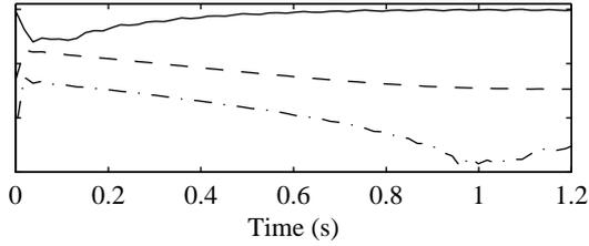
**Figure 2:** The amplitude envelope of the second harmonic of mid-plucked tanbur tone as detected in the string vibration (solid line), in acceleration of the soundboard (dashed line), and in the radiated sound (dash-dot line).
