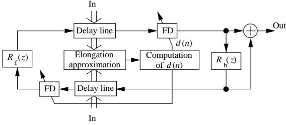
**Figure 1:** Dual-delay-line waveguide model of a string including tension modulation simulation [6, 7].
