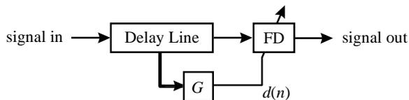
Figure 1: A general system where the input signal controls the delay parameter  $d(n)$  of a fractional delay (FD) filter. Function  $G$  computes  $d(n)$  based on the input signal sample(s).
