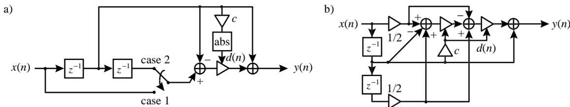
Figure 2: a) A realization structure for time-varying symmetric linear interpolator. b) A modified Farrow structure for second-order Lagrange interpolation with a signal-dependent delay parameter.
