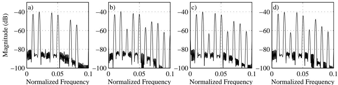
Figure 3: The magnitude spectrum of the synthetic tones produced a) without nonlinearities, b) with a switching allpass filter, c) with a switching linear interpolator, and d) with a switching second-order Lagrange interpolator.
