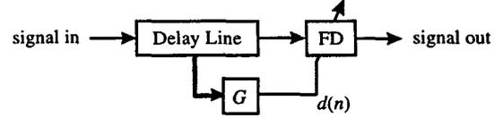
**Figure 3.** General nonlinear delay line where the delay-line signal controls the delay parameter  $d(n)$  of a fractional delay (FD) filter (adopted from [11]). Function  $G$  computes  $d(n)$  based on the contents of the delay line.
