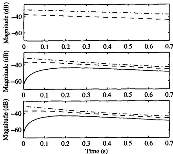
**Figure 6.** Envelopes of the first (dash-dot line), second (dashed line), and third (solid line) harmonic of synthetic tones generated by the linear (top), nonlinear single-delay-loop (middle) with  $g_p = 10.0$ , and the nonlinear single-delay-loop string algorithm with sparse power estimation ( $M = 6$ ) and  $g_p = 10.0$  (bottom).
