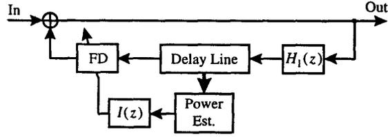
Figure 5. Single-delay-loop string synthesis model incorporating tension modulation.
