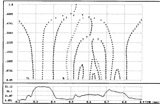
Fig. 3. An event map of a loudness function (word /kaksi). Dimensions are resolution scale vs. time.
