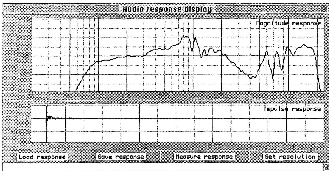
**FIGURE 1.** Measured free field magnitude response of a loudspeaker and the corresponding impulse response as shown on a typical measurement page.
