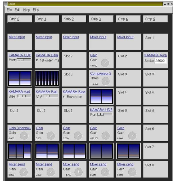
Fig. 8: Mustajuuri mixer console with two-way speech communications application.
