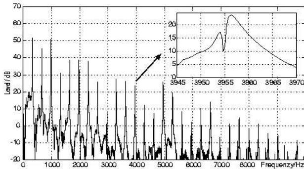
Figure 2: Spectrum of plucked string sound of a classical acoustic guitar, open string E<sub>4</sub>. Spectrum zoomed to a single partial is shown in the subplot.
