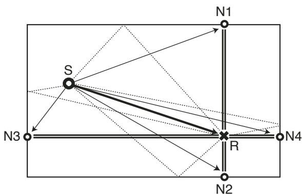
Figure 4: Simple DWN configuration in a rectangular room in the horizontal plane. S = sound source, R = receiver, and N1-N4 are scattering junctions. Thick arrow line: direct sound path; thin dotted lines: real acoustic paths of first-order reflections; and thick double axial lines: waveguides ( bi-directional delay lines). The thin solid arrow lines are for feeding junctions to approximate the first-order reflection paths.
