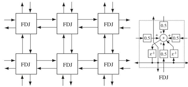
Figure 3: Left: part of a rectilinear 2-D FDTD mesh structure. Bi-directional delay-free connections link the junctions (square blocks) and the memory  $z^{-2}$  is a part of the junction. Right: computation of an FDTD junction.
