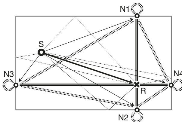
Figure 5: DWN configuration in a rectangular room with added non-axial waveguides (dotted double lines) and loading of nodes for losses and dispersion/diffusion (circular dotted double lines).
