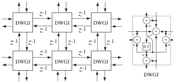
Figure 2: Left: part of a rectilinear 2-D waveguide mesh structure. Bi-directional unit delays  $z^{-1}$  connect scattering junctions (square blocks). Right: computation of a DWG scattering junction, Eq. (1).
