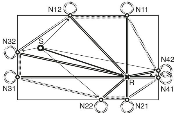
Figure 6: A DWN structure where secondary waveguides (N12-R-N22, N32-R-N42) are added to correct arrival directions of first-order reflections. For improved cross-modes and reflections, all nodes are connected into a polygon path (dotted double lines). Losses and dispersion/diffusion at the walls is increased by circular connections at each node (circular dotted double lines).
