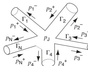
Figure 1: A scattering junction of connected acoustic tubes. Traveling pressure waves are denoted by '+' for incident and by '-' for scattered wave components.
