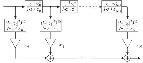
Figure 2: The Kautz filter. For  $z_i = 0$  in (3) it degenerates to an FIR filter, for  $z_i = a$ ,  $-1 < a < 1$ , it is a Laguerre filter where the tap filters can be replaced by a common pre-filter.
