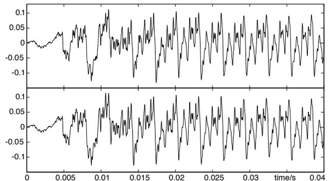
Figure 5: The first 40 ms of the original plucked string signal (top) and the response of the Kautz model (bottom).
