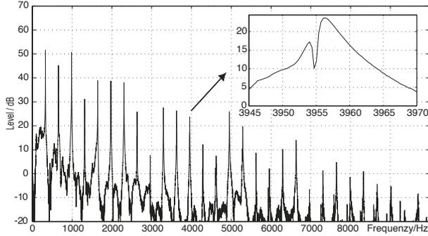
Figure 1: Spectrum of plucked string sound of a classical acoustic guitar, open string E<sub>4</sub>. Spectrum zoomed to a single partial is shown in the subplot.
