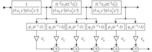
Figure 3: A real Kautz filter [6], where the normalizing coefficients  $\{p_i, q_i\}$  can be absorbed into  $\{c_i\}$ .
