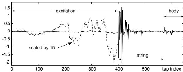
Figure 7: Tap coefficients of the Kautz model for different parts of the model. The FIR part is amplified by factor 15 as the dotted line.
