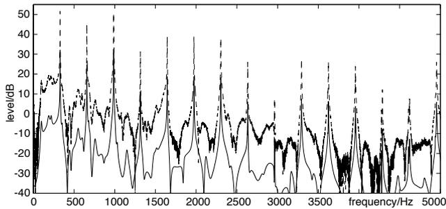
Figure 6: Spectra of the original (upper, dotted) and the resynthesized guitar sound (lower, solid) for 0–5 kHz. The synthesized spectrum is lowered by 20 dB.
