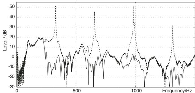
Figure 4: Low-frequency spectrum for the original plucked signal spectrum (dashed line) and the residual spectrum when the FZ-ARMA modeled string modes are removed (solid line).
