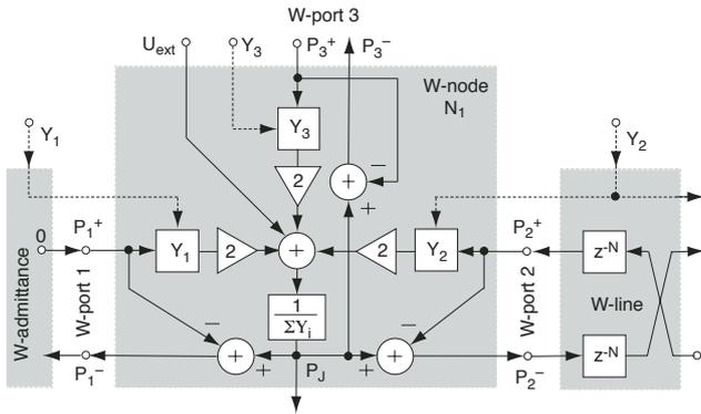
Figure 1: A 3-port parallel scattering junction for acoustic pressure waves. Port 1 (left) is terminated by admittance  $Y_1$ , port 2 (right) is connected to a delay-line, and port 3 (top) is not connected.
