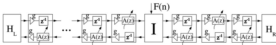
Figure 7: A nonlinear DWG string. The string consists of allpass filters, denoted  $A(z)$ , connected via unit delays for avoiding delay-free loops.  $H_L$  and  $H_R$  denote loop filters simulating the frequency-dependent losses and  $g$  is a scaling coefficient for modeling frequency-independent losses.  $F(n)$  represents the excitation force signal applied on the string.
