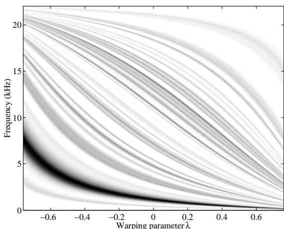
Figure 5: Body simulation filter’s magnitude response as a function of the warping parameter  $\lambda$ . The tone values indicate the magnitude of the guitar body resonances. Darkest colors represent the strongest resonances.
