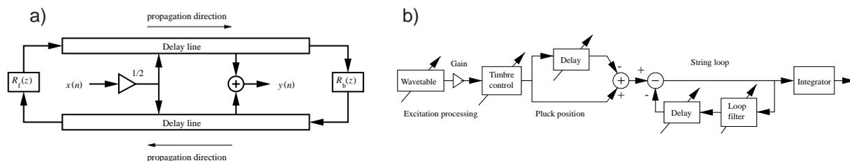
Figure 1: Reduction of a dual delay line digital waveguide model (a) into a single delay loop model (b). Filters  $R_f(z)$  and  $R_b(z)$  model wave reflection at string terminations.  $x(n)$  is pluck excitation and  $y(n)$  pickup output (bridge output in the acoustic guitar). The single delay loop model (b) consist of wavetable excitation, timbre and pluck position filters, string loop with delay and attenuation (loop filter) controls, and an integrator.
