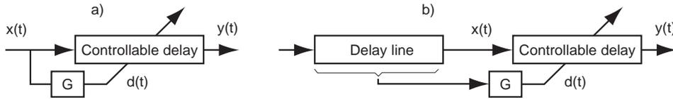
Figure 3: Controllable delays as approximations for passive nonlinearity: (a) Input signal is used through transform  $G$  to control delay and (b) delay control signal comes from another part of the system, in this example it is computed from a distributed time-varying property of a string delay line.
