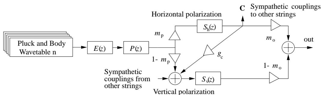
Figure 2: A dual-polarization string model for the acoustic guitar including sympathetic couplings [17].  $S_h(z)$  is horizontal and  $S_v(z)$  vertical submodel.  $C$  is matrix of sympathetic couplings,  $m_p$  and  $m_o$  control the coupling of the submodels,  $P(z)$  is a plucking point filter, and  $E(z)$  pluck tone control filter for wavetable excitation variation.
