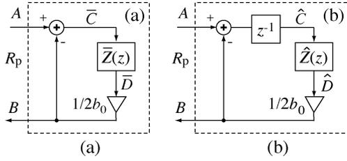
Fig. 10. One-port block made of general impedance according to (25) with subfilter  $\tilde{Z}(z)$  or  $\hat{Z}(z)$ .
