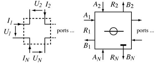
Fig. 4. Series adaptor: (left) connection for  $K$ -variables, (right) corresponding WDF symbol for wave variable, including reflection-free port  $N$  marked by signal terminal symbol  $T$ .
