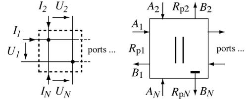
Fig. 2. Parallel adaptor: (left) connection for K-variables, (right) corresponding WDF symbol for wave variable, including reflection-free port  $N$  marked by signal terminal symbol  $T$ .
