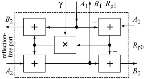
Fig. 3. Three-port parallel adaptor with a reflection-free port.
