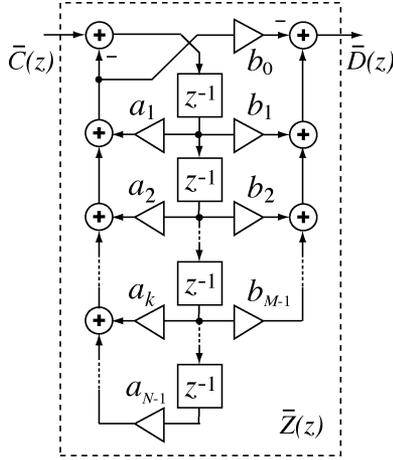
Fig. 12. Subfilter  $\bar{Z}(z)$  according to (25) and Fig. 10(a) to realize a wave port for impedance  $Z(z)$  as specified by a rational expression in (32).
