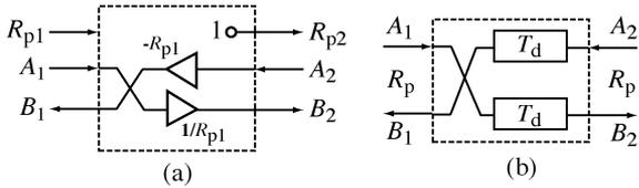
Fig. 9. Two-port WDF elements: (a) dualizer and (b) delay-line.
