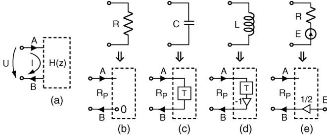
Fig. 1. Definition of basic WDF one-port elements. (a) A generic one-port, (b) resistor:  $R_p = R$ , (c) capacitor:  $R_p = T/2C$ , (d) inductor:  $R_p = 2L/T$ , (e) voltage source:  $R_p = R$ , where  $C$ ,  $L$ , and  $R$  are physical capacitance, inductance, and resistance, respectively, and  $T$  is unit delay.
