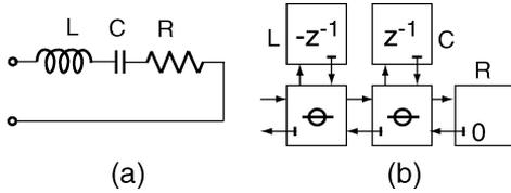
Fig. 7. (a) Series LCR circuit and (b) its WDF realization using three-port series adaptors.
