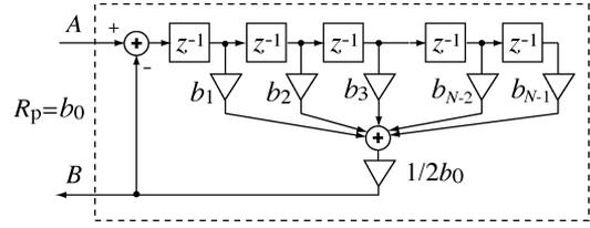
Fig. 11. One-port block with wave port for a given polynomial impedance of (28) to realize the reflectance of (31) and port resistance of (30).
