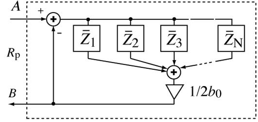
Fig. 13. One-port block with wave port for impedance given as a combination of subfilters  $\bar{Z}_k(z)$  for series connection of impedances.
