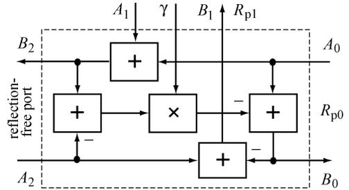
Fig. 5. Three-port series adaptor with a reflection-free port.
