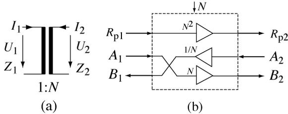
Fig. 8. (a) Ideal transformer and (b) its WDF realization.
