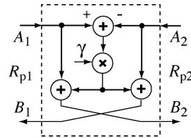
Fig. 6. One-multiplier realization of two-port adaptor.
