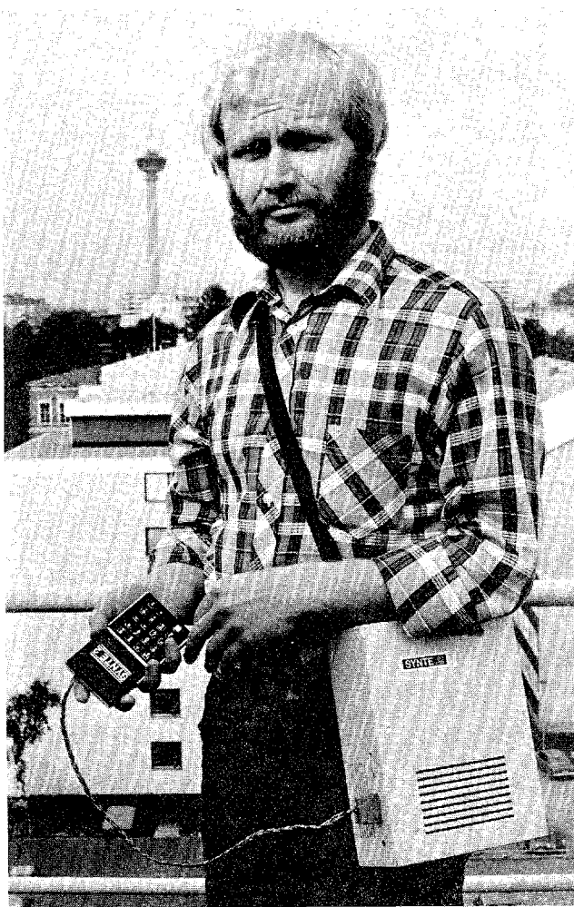
Fig. 2. Prototype of the speaking machine for the speech impaired
