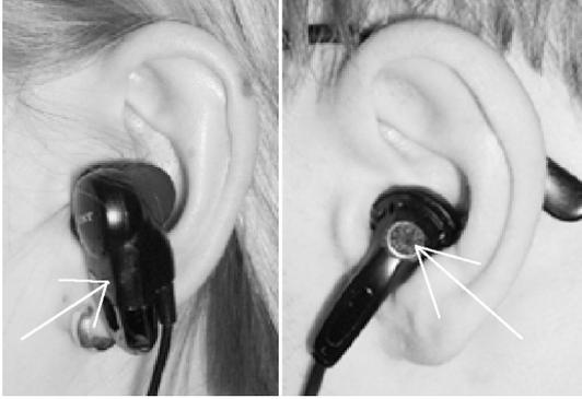
Fig. 4: Two different types of headsets used in MARA applications. The arrows point at the microphones.
