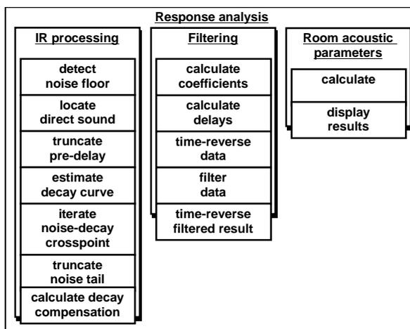
Fig. 4. Response processing and filtering prior to standard room acoustical analysis with the IRMA measurement system.
