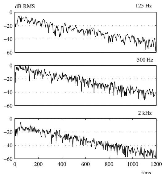
Fig. 8. Energy-time curves for the 125, 500, and 2000 Hz octave bands.
