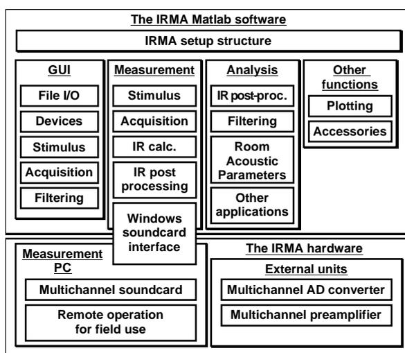
Fig. 2. A functional layout of the IRMA measurement system.
