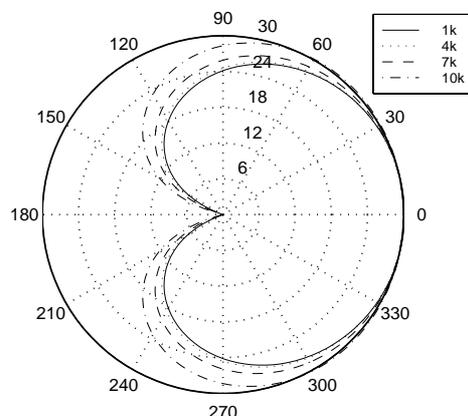
Fig. 5. Polar dB magnitude plots of  $p'(t, \omega, 0)$  with  $d = 10$  mm on four different frequencies.
