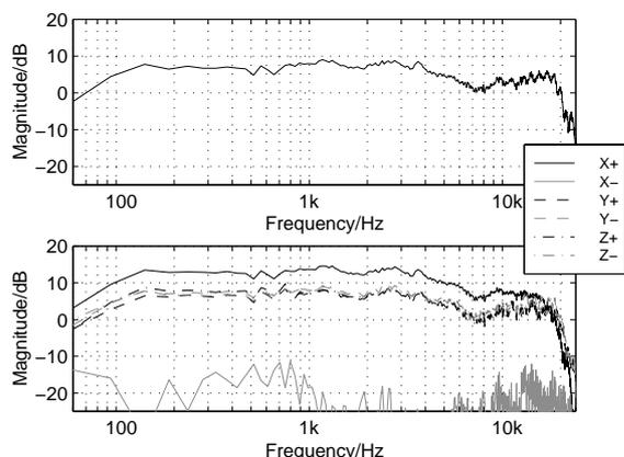
Fig. 6. Top: Magnitude response of the loudspeaker used as a sound source. Bottom: Responses of 6 cardioids pointing to different directions.
