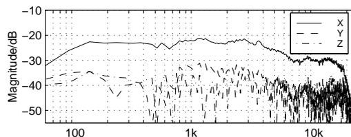
Fig. 7. Sound intensity of the loudspeaker measured in an anechoic chamber.
