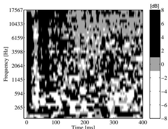
Fig. 10. An example analysis of lateral energy flow. Black areas are obtained when the signal from the left side cardioid microphone is dominating, and white areas for the right side respectively.
