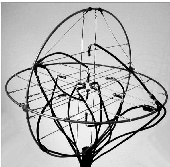
Fig. 3. A picture of the 3-D microphone probe.
