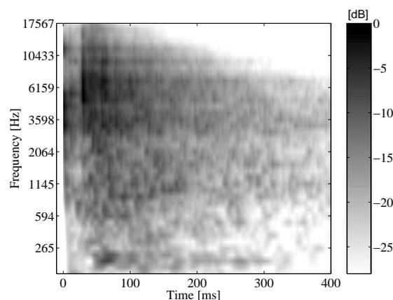
Fig. 9. An example of auditorily motivated analysis on the studied impulse response. Both the source and the microphone used exhibit omnidirectional directivity patterns.
