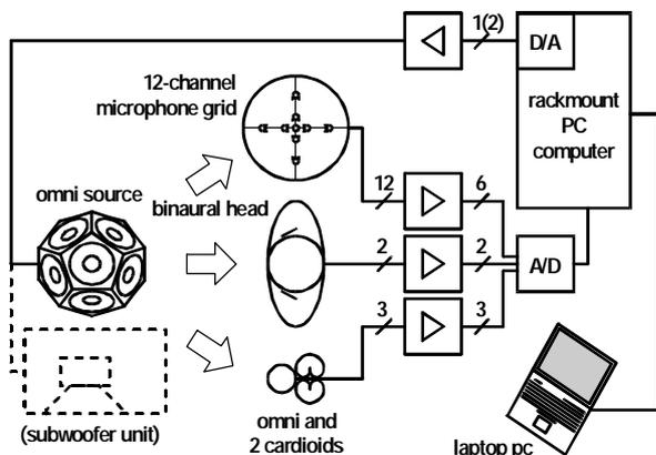
Fig. 1. The measurement system hardware layout.
