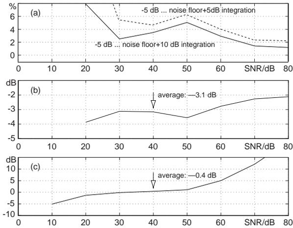
Fig. 5: Decay parameter estimation errors for the Lundeby *et al.* method as a function of SN-ratio: (a) decay time estimation error percentage with truncated Schroeder integration but without noise compensation, (b) initial level estimation error in dB, and (c) noise floor estimation error in dB.
