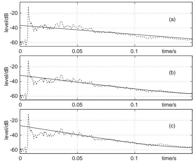
Fig. 6: Decay-plus-noise model fitting by nonlinear optimization to a room impulse response: (a) fitting range includes initial delay, transient phase, and decay, (b) fitting includes transient phase and decay, and (c) fitting includes only the decay phase.
