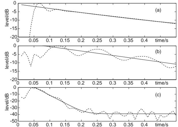
Fig. 9: Examples of modal decay matching for harmonic components of a guitar string: (a) regular decay after initial transient, (b) strongly beating decay (double mode), and (c) fast decay that reaches the noise floor. Dotted line: measured envelope, solid line: optimized fit.
