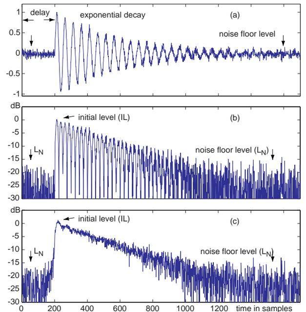
Fig. 1: (a) Single mode impulse response (sinusoidal decay) with initial delay and additive measurement noise. (b) Absolute value of response on the dB scale to illustrate the decay envelope. (c) Hilbert envelope, otherwise same as (b).
