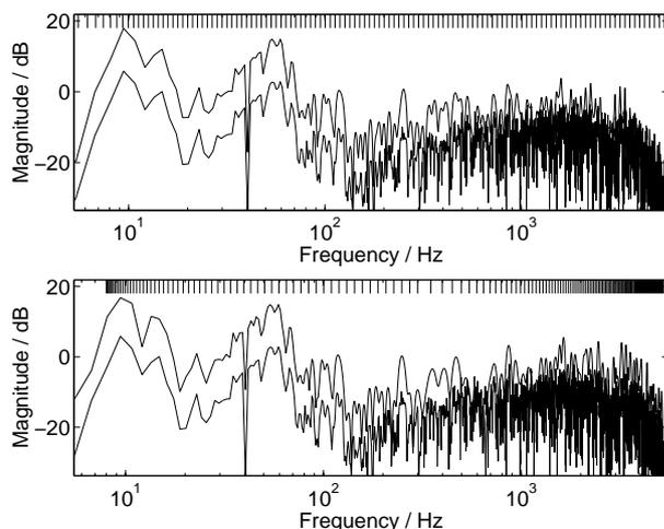
Fig. 9: Two Kautz models plotted with upward offset to the target magnitude response, Kautz model orders 236 (top) and 320 (bottom), with pole pair positions indicated by vertical lines.
