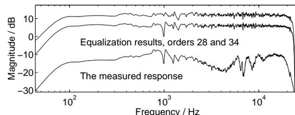
Fig. 4: Kautz equalization results for orders 28 and 34, with pruned BU-poles.
