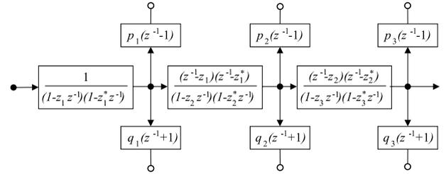
Fig. 2: One realization for producing real Kautz filter tap-output responses defined by a sequence of real complex conjugate pole pairs. The transversal all-pass backbone of Fig. 1 is restored by moving the denominator terms one step to the right and compensating for the change in the tap-output filters.
