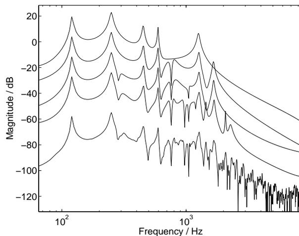
Fig. 17: Displayed with offset from top to bottom, Kautz models of orders 10, 16, 20 and 40, and the target magnitude response.
