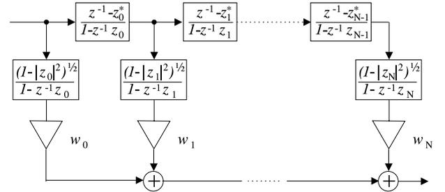
Fig. 1: The Kautz filter. For  $z_i = 0$  in (1) it degenerates to an FIR filter and for  $z_i = a$ ,  $-1 < a < 1$ , it is a Laguerre filter where the tap filters are replaced by a common pre-filter.
