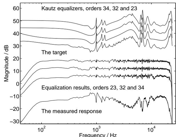
Fig. 5: Kautz equalizers and equalization results for orders 23, 32 and 34, with combinations of manually tuned and BU-generated poles.
