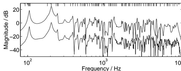
Fig. 19: Magnitude responses for a 160th order Kautz model of another acoustic guitar body impulse response, displayed together with upward offset.
