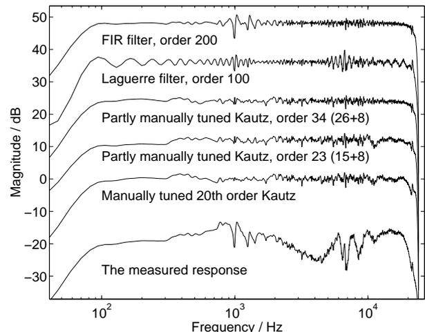
Fig. 7: Comparison of FIR, Laguerre, and Kautz equalization results.
