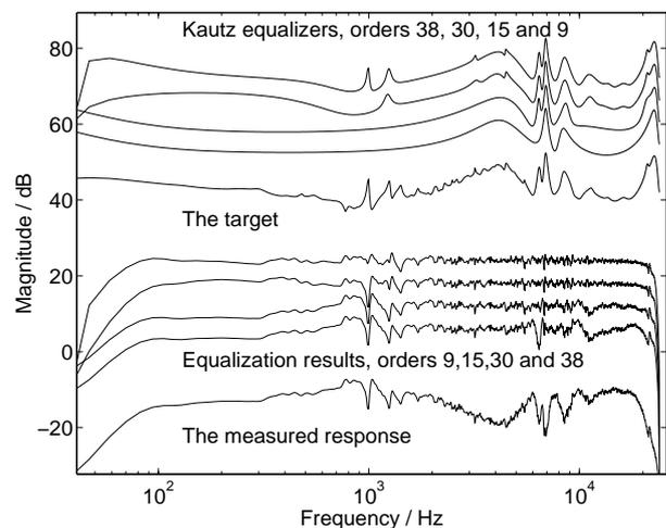
Fig. 3: Kautz equalizers and equalization results for orders 9, 15, 30 and 38, compared to the measured loudspeaker response and the equalizer target response.
