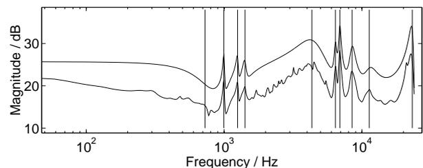
Fig. 6: Manually tuned 20th order Kautz equalizer and target responses, with lines indicating pole pair positions.
