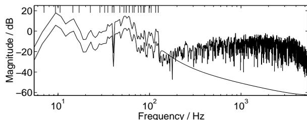
Fig. 11: A 50th order Kautz model for accurate modeling of the lowest frequencies.
