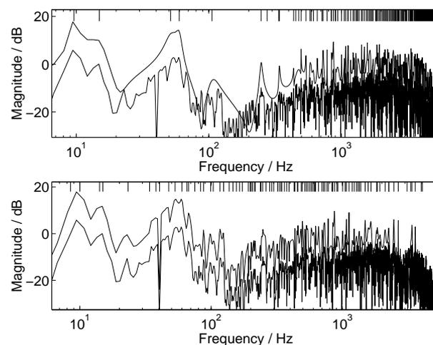
Fig. 10: Kautz models with BU-poles, with filter order 300 (top) and by warping and back-mapping at the filter order 200 (bottom).
