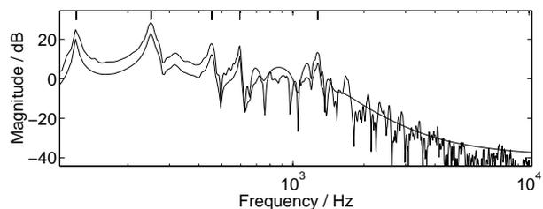
Fig. 14: Displayed with upward offset, magnitude responses of the target and a 80th order Kautz model.
