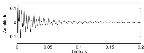
Fig. 18: The impulse response of a 10th order Kautz filter modeling the response in Fig. 13.
