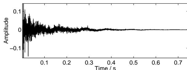
Fig. 8: A measured room impulse response.
