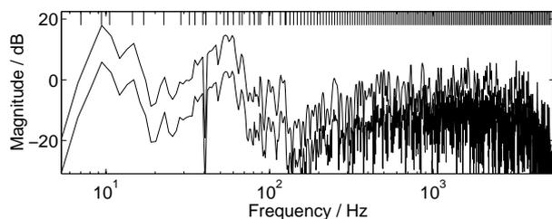
Fig. 12: A 326th order Kautz model produced by adding poles (indicated by vertical lines) to the pole set of the model in Fig. 11.
