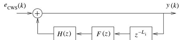
Fig. 1: Block diagram of the String Model
