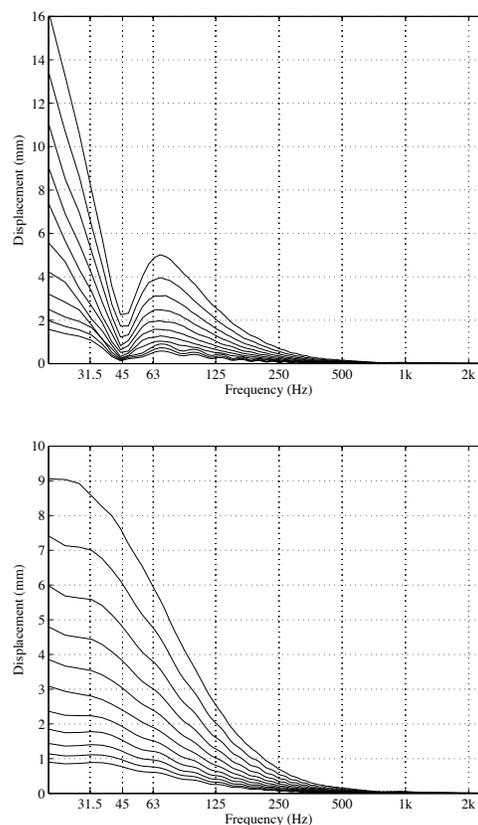
**Fig. 13:** Displacement (peak-to-peak level) as a function of frequency with open (upper) and with closed (lower) reflex port.
