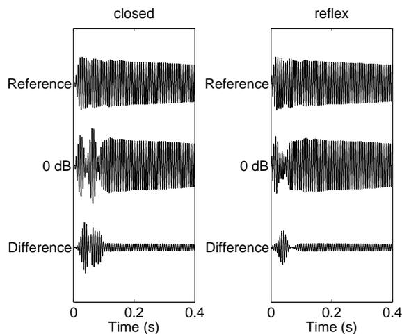
**Fig. 9:** Envelopes of the bandlimited (center frequency of the band 199 Hz) 'ebass' test tones in closed (left) and reflex (right) enclosures. The response levels are matched. The bottom envelope is the difference of the reference tone and 0 dB tone envelopes.
