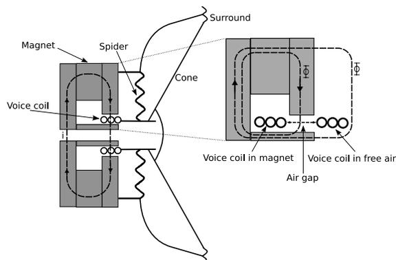
Fig. 1: Sectional view of the dynamic driver.
