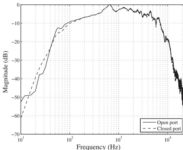
**Fig. 3:** Frequency responses for the loudspeaker with open (solid) and closed (dashed) reflex port.
