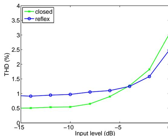
**Fig. 8:** Total harmonic distortion of the 114 Hz sinusoidal tone in closed and reflex enclosures. Input level 0 dB is the input level of the original tone.
