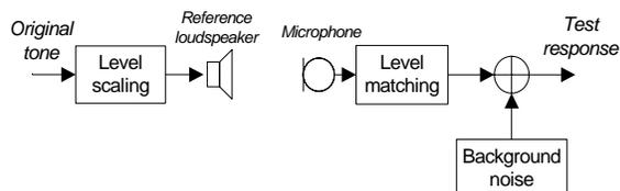
**Fig. 6:** Block diagram of the test tone production system.
