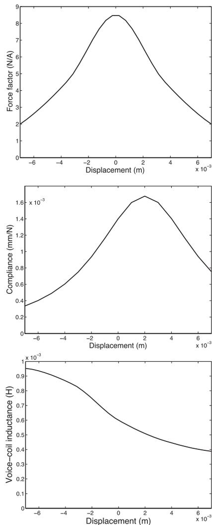
**Fig. 2:** Nonlinear a) force factor b) compliance and c) inductance as a function of displacement. Curves have been interpolated using data from [13].
