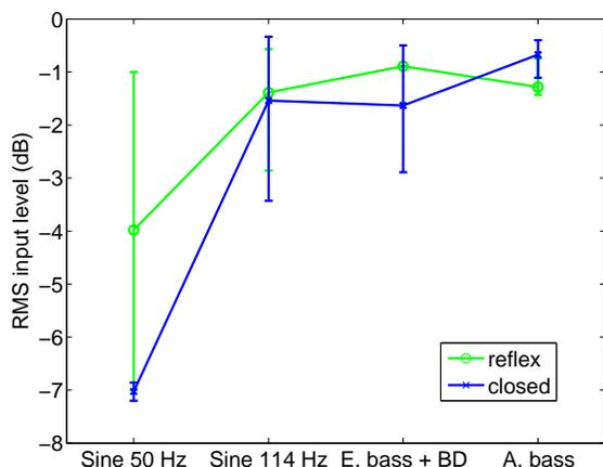
**Fig. 15:** Limits of audibility of distortion for the four test tones in closed (blue line with crosses) and reflex (green line with circles) enclosures based on the listening experiments. Notice the large variance of the 'sine50' case.
