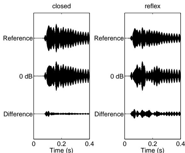
**Fig. 10:** Envelopes of the bandlimited (center frequency of the band 649 Hz) 'abass' test tones in closed (left) and reflex (right) enclosures. The response levels are matched. The bottom envelope is the difference of the reference tone and 0 dB tone envelopes.
