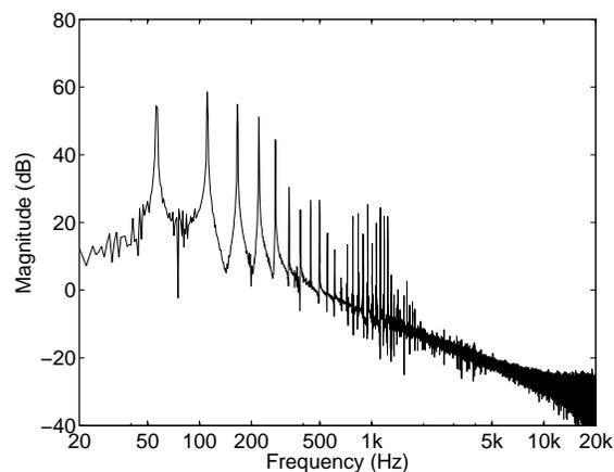
**Fig. 4:** Spectrum of the 'ebass' test tone including electric bass and bassdrum sounds.
