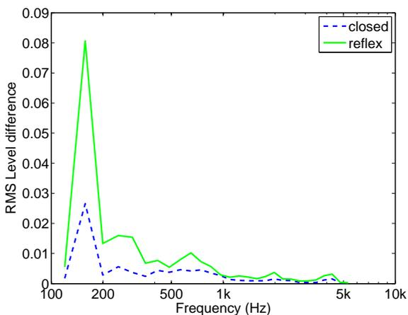
**Fig. 12:** RMS level differences at ERB frequency bands for 'abass' and test tone in closed (dashed blue line) and reflex (solid green line) enclosures when envelopes of signals with input levels 0 dB and -10 dB are compared.
