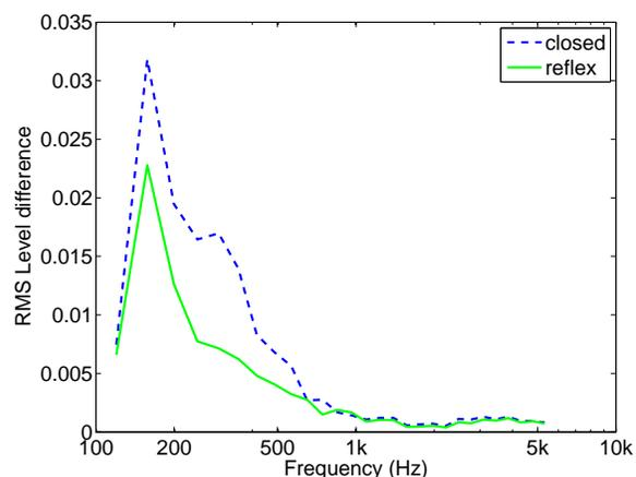
**Fig. 11:** RMS level differences at ERB frequency bands for 'ebass' test tone in closed (dashed blue line) and reflex (solid green line) enclosures when envelopes of signals with input levels 0 dB and -10 dB are compared.
