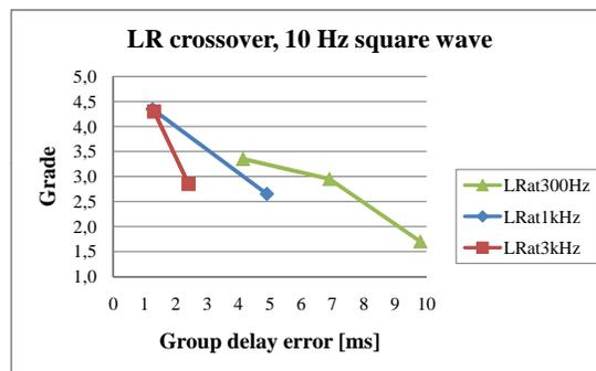
**Fig. 6:** Grade as a function of group delay error for 10 Hz square wave signal with L-R crossovers. There is no delay between drivers. The graphs behave regularly, descending as the group delay error increases.
