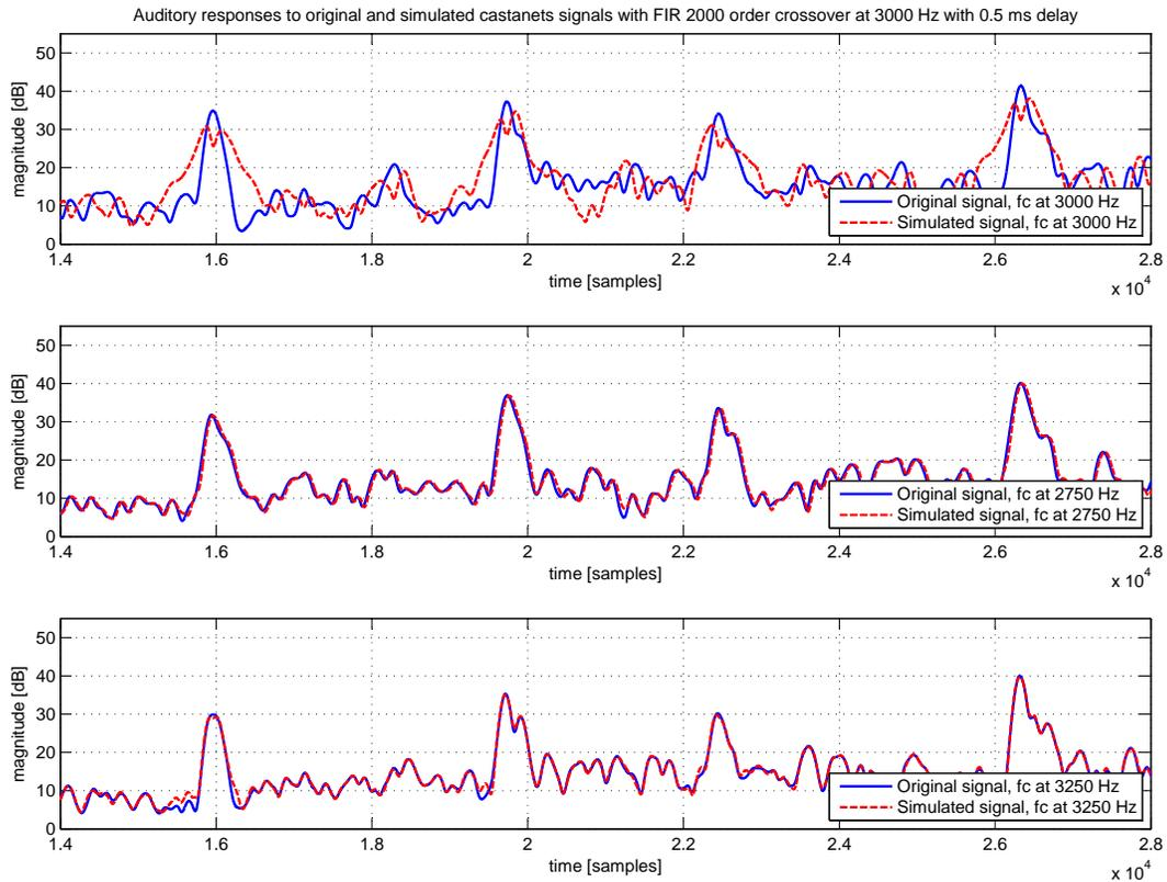
**Fig. 20:** Auditory analysis responses to castanet signal with 2000th order FIR crossover filter on three adjacent auditory channels: 3000 Hz (crossover channel, top subplot), 2750 Hz (lower channel, middle subplot), and 3250 Hz (upper channel, bottom subplot). The delay between drivers is 0.5 ms. On the auditory channel corresponding to the crossover frequency, crossover simulated signal response is flattened from the top, and also clearly spread in time. The average grade was 2.3.
