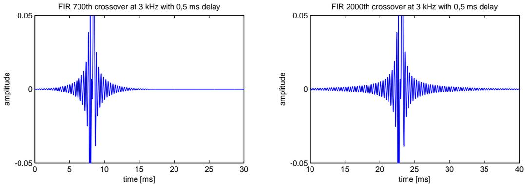
**Fig. 12:** Comparison of impulse responses of 700th order FIR (left) and 2000th order FIR (right) crossovers at 3 kHz in an off-axis position (the delay between drivers is 0.5 ms) to demonstrate the ringing phenomenon. Notice how the duration of ringing grows with increasing filter order.
