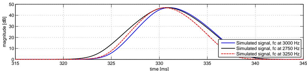
**Fig. 17:** Auditory analysis responses to 10 Hz square wave signal with 32th order L-R crossover filter on three auditory channels without the original signal: 3000 Hz (crossover channel), 2750 Hz (lower channel), and 3250 Hz (upper channel). The delay between drivers is 0 ms. Notice how the responses differ in time due to changing group delay of the L-R crossover, producing audible phase errors.
