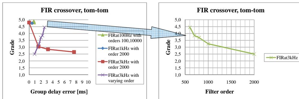
**Fig. 11:** Grade as a function of group delay error for the tom-tom with FIR crossovers. The last series in the left subplot is an FIR with varying order, and strange behaviour is again noticed. It is extracted into the right subplot to show the effect of the filter order.
