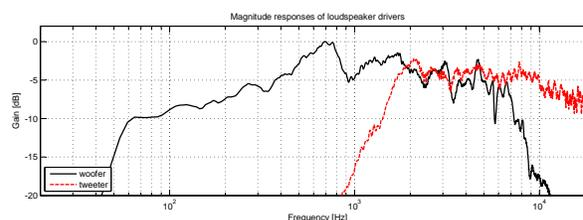
**Fig. 1:** Magnitude responses of drivers of the loudspeaker that was used in the real loudspeaker experiment.
