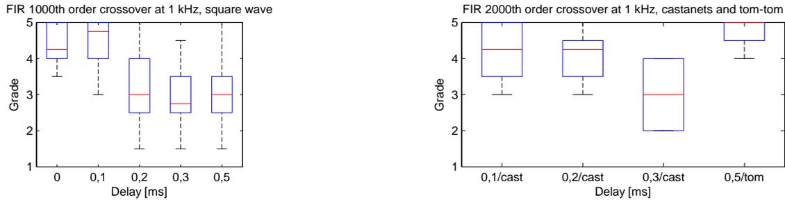
**Fig. 2:** Combined results of the listening test for FIR crossovers at 1 kHz. Square wave is susceptible to clearly audible degradation with 0.2 ms delay, castanets with 0.3 ms delay, while tom-tom receives high grade even with 0.5 ms delay.
