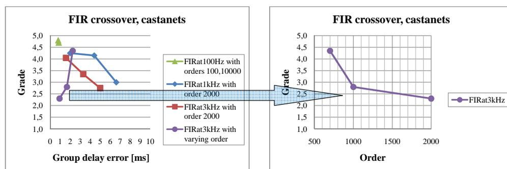
**Fig. 10:** Grade as a function of group delay error for the castanets with FIR crossovers. The last series in the left subplot is a FIR with varying order, and strange behaviour is noticed. It is extracted into the right subplot to show the effect of the filter order.
