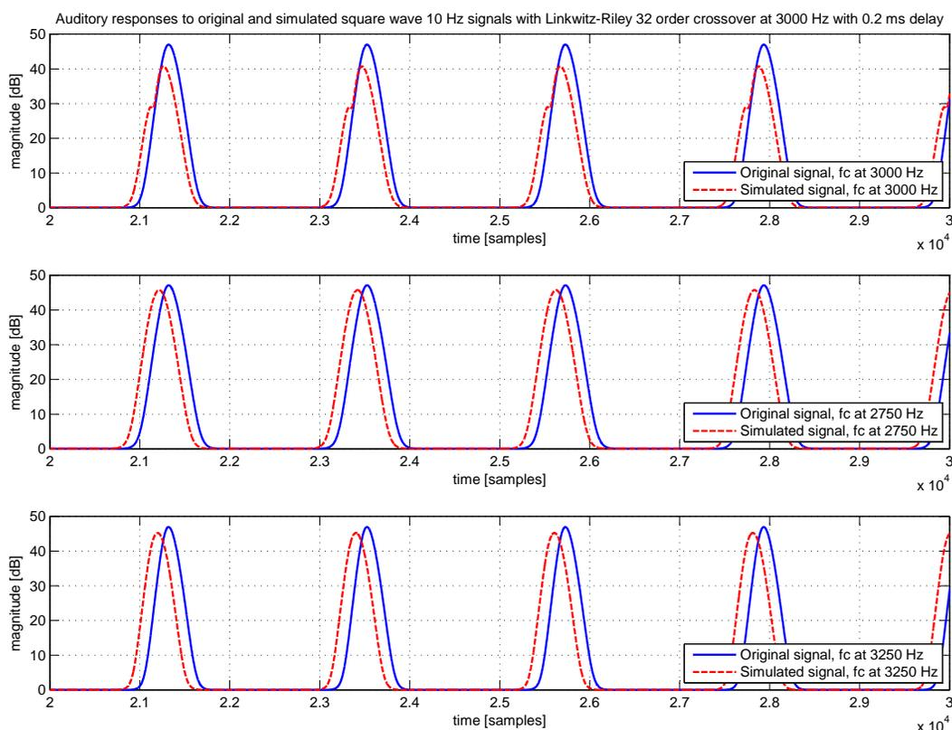
**Fig. 18:** Auditory analysis responses to 10 Hz square wave signal with 32th order L-R crossover filter off-axis on three adjacent auditory channels: 3000 Hz (crossover channel, top subplot), 2750 Hz (lower channel, middle subplot), and 3250 Hz (upper channel, bottom subplot). The delay between drivers is 0.2 ms. On the auditory channel corresponding to the crossover frequency, crossover-simulated signal response shows a bump on the left side. The average grade was 3.1.
