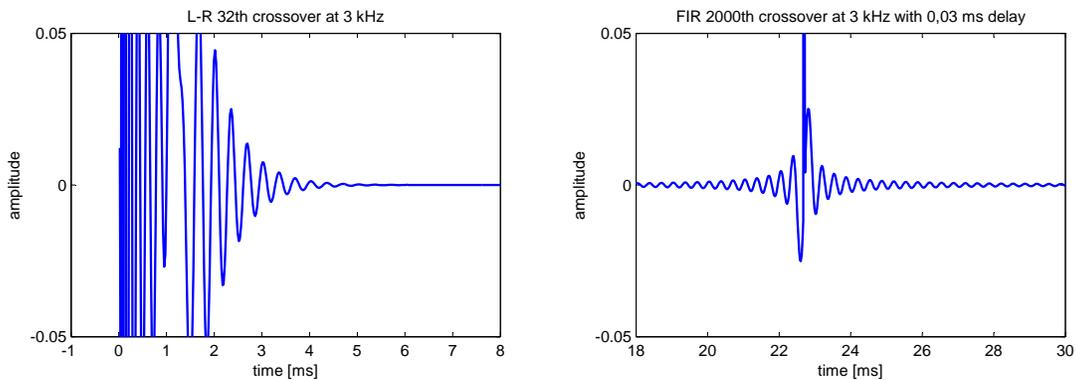
**Fig. 13:** Comparison of impulse responses of 32th order L-R (left) and 2000th order FIR (right) crossovers to demonstrate the ringing phenomenon. Notice the asymmetry in ringing of L-R's vs. the symmetry of FIR's. The impulse responses are closely zoomed to illustrate the phenomenon better.
