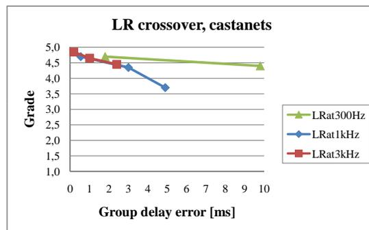
**Fig. 7:** Grade as a function of group delay error for castanets with L-R crossovers. There is no delay between drivers. As with square wave, the slopes are descending, though not as abruptly.
