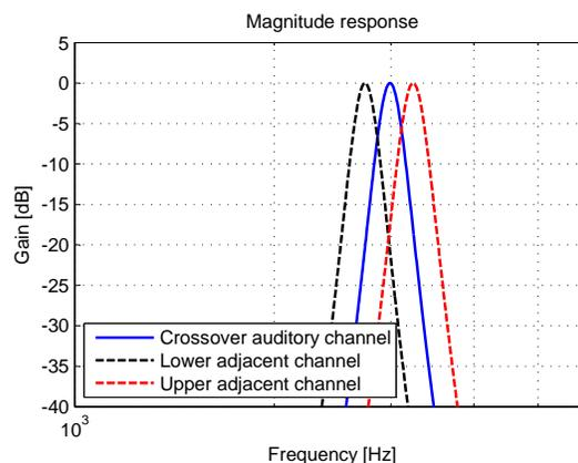
**Fig. 15:** Magnitude responses of used filterbank's three channels. The main channel's center frequency corresponds to the crossover frequency (here 3000 Hz). The lower (center frequency 2750 Hz) and upper (center frequency 3250 Hz) adjacent channels are also plotted. The -6 dB bandwidth is roughly 260 Hz.
