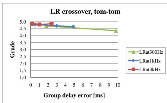
**Fig. 8:** Grade as a function of group delay error for tom-tom with L-R crossovers. There is no delay between drivers. As with the two other signals, the slopes are descending, but the rate is even smaller.
