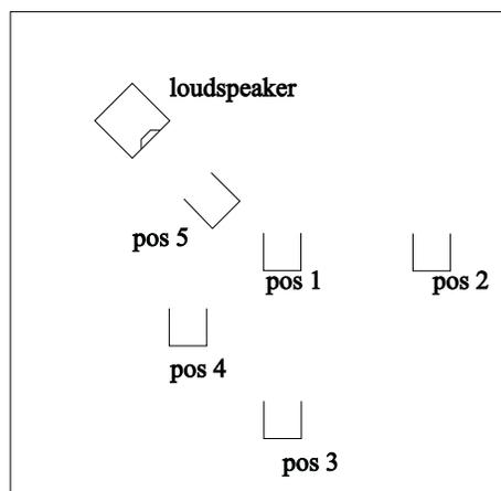
**Fig. 5:** Listening positions 1-5 of the real loudspeaker experiment. Loudspeaker was placed as the left channel in stereo listening (for position 1).
