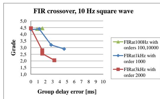
**Fig. 9:** Grade as a function of group delay error for the square wave with FIR crossovers. The graphs behave regularly, descending as the group delay error increases.
