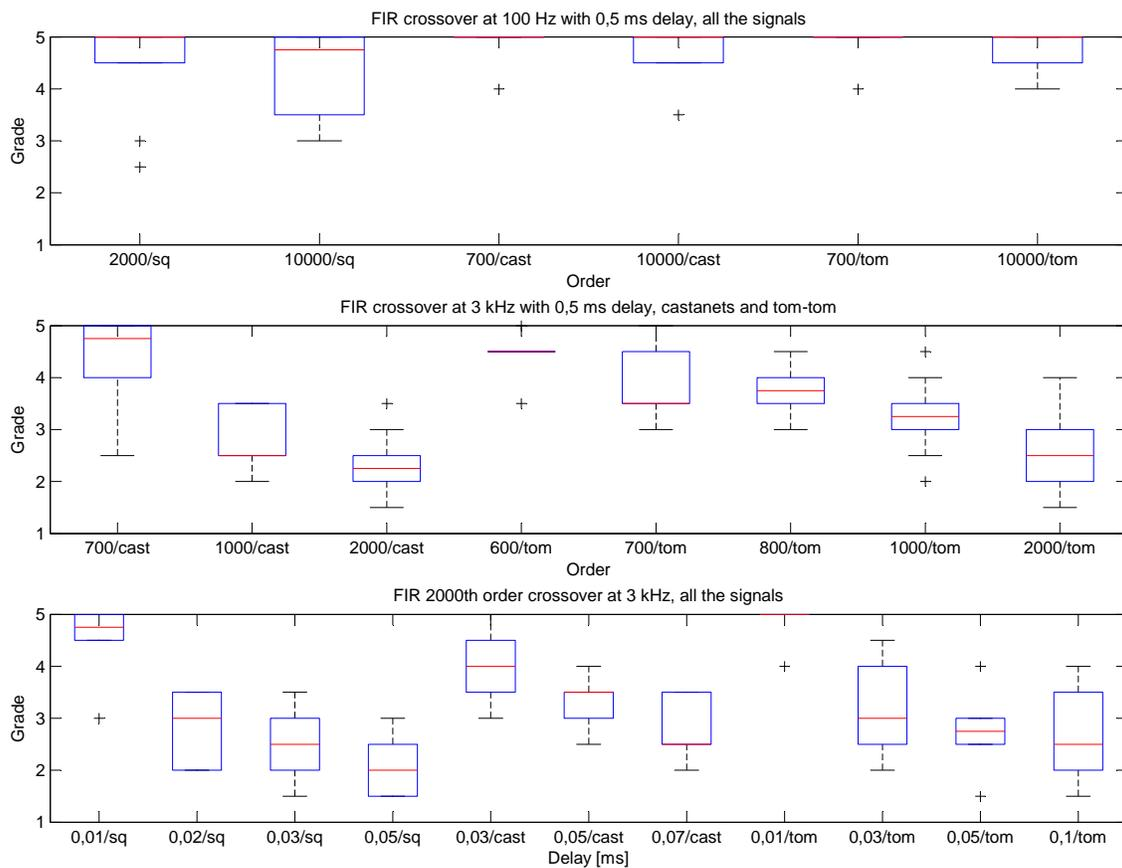
**Fig. 3:** Combined results of the listening test for FIR crossovers. Top: At 100 Hz no considerable degradations are perceived. Middle: At 3 kHz with long delay the grades seem to decrease after order or 600-700. Bottom: At 3 kHz with varying delay, even small delays seem to degradate the signals in an audible way.
