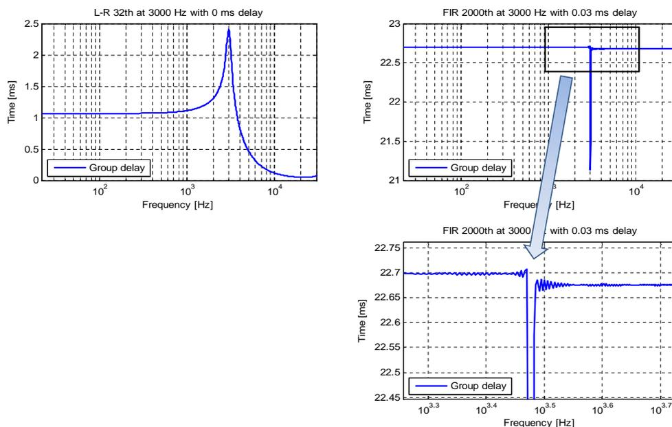
**Fig. 14:** Group delay graphs of L-R (left) and FIR (right) crossovers. Notice the abrupt changes of FIR crossover's group delay around the crossover frequency in the zoomed subplot (bottom).
