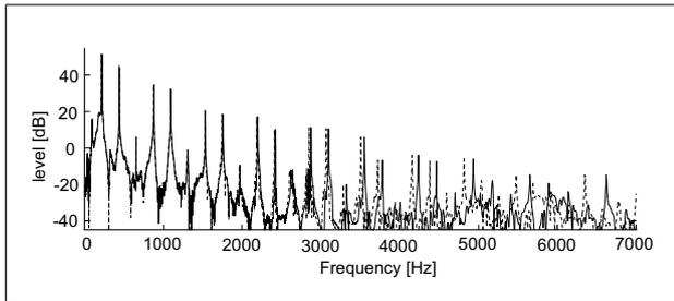
Figure 3. Example of an inharmonic plucked string spectrum (solid line) and a harmonic resynthesized version of it (dashed line).
