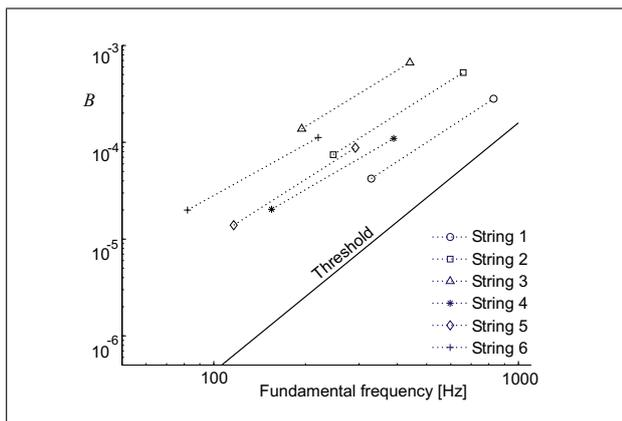
Figure 1. Perception thresholds from [3] (solid line) versus inharmonicity coefficients  $B$  for frets 0-17 of each string as a function of fundamental frequency.
