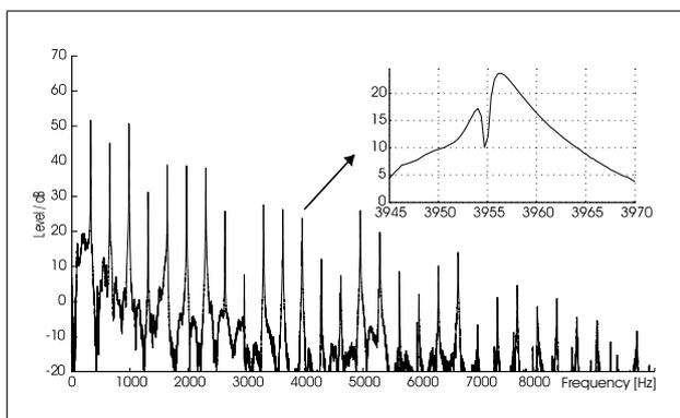
Figure 2. Spectrum of plucked string sound of a classical acoustic guitar, open string  $E_4$ . Spectrum zoomed to a single partial is shown in the subplot.
